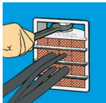
7 Tighten the compression plate bolt until the tongue of the E-STG-1 slides into position around the bolt (32 mm maximum from the inside of the frame to the top of the compression plate).
