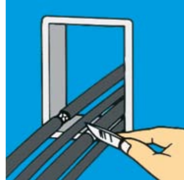
2 Pull cables to final position. Mark cable 30 mm from front edge of frame. Remove cable sheath 5 mm on either side of the line.
