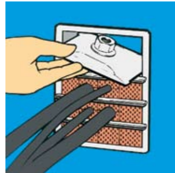
5 Before the final row of blocks, the compression plate is installed. Alternatively, the E-PTG Presswedge can be fitted.
