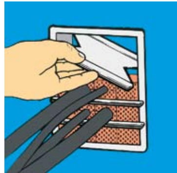
4 Position the stayplates between each layer of insert blocks.
